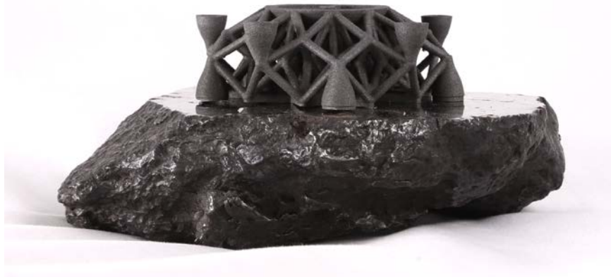
Figure 14. Spacecraft Propulsion Structure 3D Printed from Actual Asteroid Material
