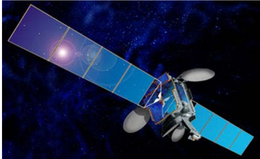
Figure 7. Example of a Communications Satellite Showing Three Antennas Customized for Specific Markets Defined by Their Geographic Location
