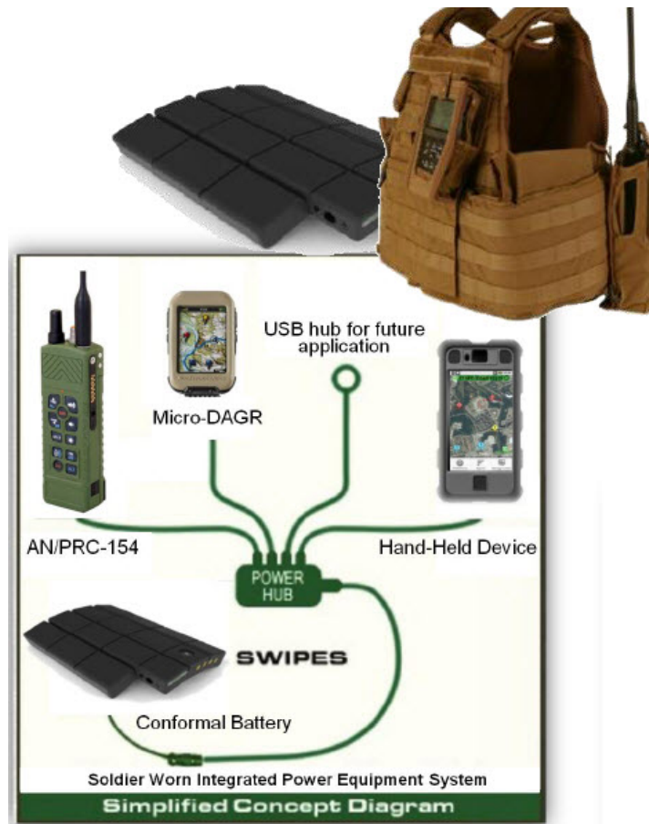
Figure 8. Diagram and Photo of SWIPES and the Accompanying Conformal Battery
