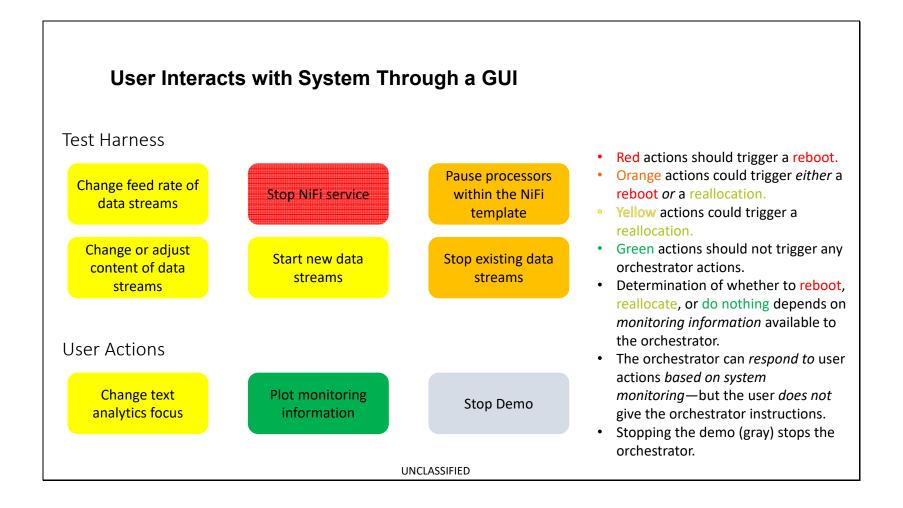
This diagram represents all the actions that are available through the GUI, including actions designed to disrupt the activity of the NiFi system. The test harness actions are designed to mimic events that would be occurring in the environment, outside the control of the system user. In an operational context, these would be the events that a resilience engineering system would need to react to.
