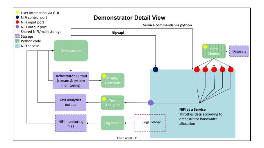
This schematic is a wiring diagram representing the full system. The full system runs inside a docker container that can be hosted on a Linux machine or Amazon Web Services node. The goal is to show how the orchestrator and other python code components interact with file storage and the NiFi service.
