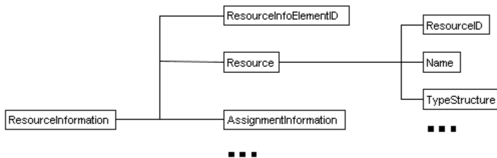
Figure 2-1. UICDS ResourceInformation Structure
