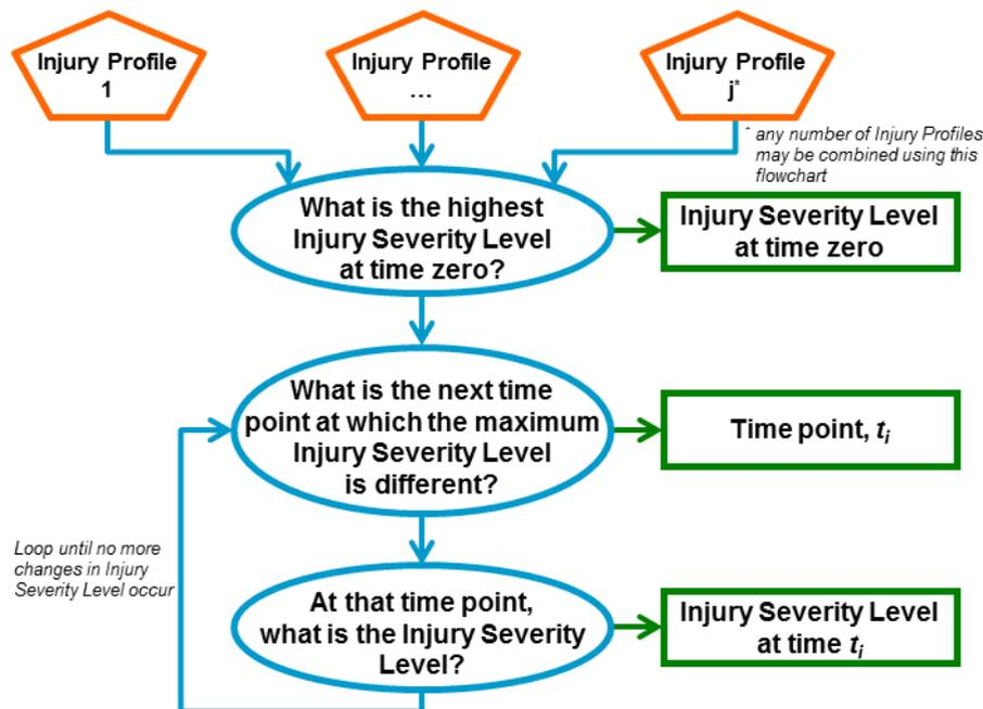
Figure 4-1: Flowchart for Generation of Composite Injury Profiles
