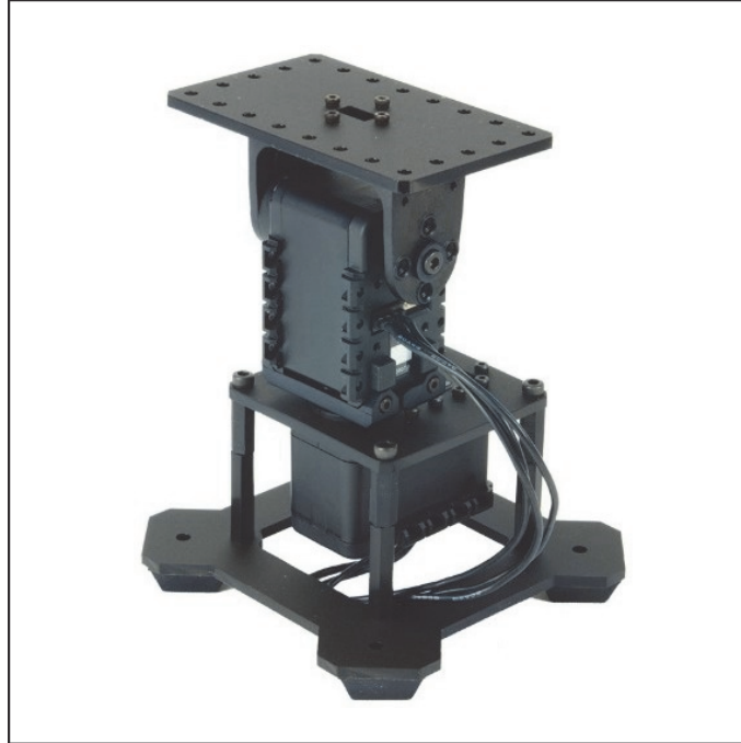
Figure 2. The PhantomX Pan Tilt Stand that forms the base of the ONT, with two installed AX-12 servomotors. 3
