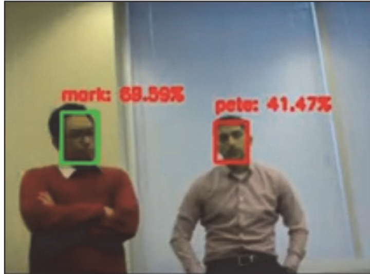
Figure 10. The field of view of the webcam, demonstrating identification of friendly (green) and hostile (red) faces
