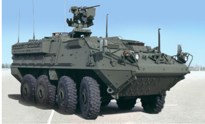
Figure 1. The Infantry Carrier Vehicle (ICV) serves as the base vehicle for eight additional system configurations. SOURCE: www.sbct.army.mil .
