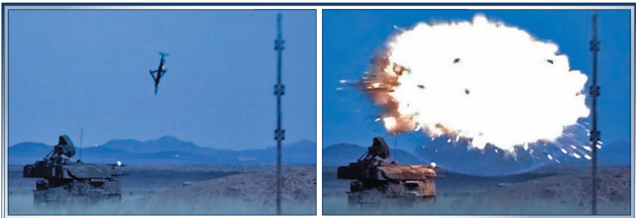
A Small Diameter Bomb attacks an actual threat air defense vehicle using the bomb's airburst function. IDA is evaluating many of the nation's most important munitions, and assessing the effectiveness of weapons against realistic targets is an important part of our munition evaluations. Traditionally, munition live-fire tests were conducted using a static warhead. While this procedure provided some detailed information, it did not replicate the dynamics of an actual flight test. IDA has encouraged the Services to move away from static tests as much as possible and include realistic targets in planned flight tests. This can reduce the program's overall test cost while providing more realistic assessments.
