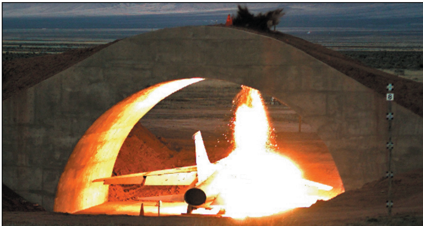
A Small Diameter Bomb is fired against a U.S. A-7 aircraft in a simulated shelter. The shelter's wall-thickness and cross-section are representative of an actual threat shelter. A major factor in the LFT&E testing is ensuring that weapon systems are tested against realistic threat targets or surrogates.
