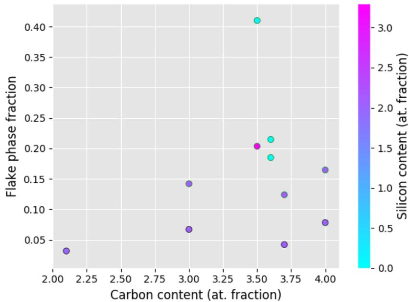
**Figure 10. Estimated flake phase fraction based on n-point statistic image processing as a function of C content. Points outlined in black are from unetched images. Data point color corresponds to Si content.**
