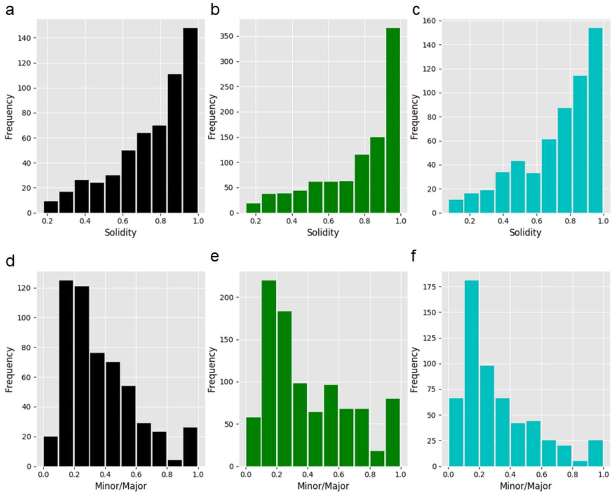
**Figure 9. Example histograms for graphitic flake solidity and minor/major axis ratio for three images of grey cast iron. From left to right, the compositions are: (a,d) 2.1% C, 2.0% Si (b,e) 3.0% C, 2.1% Si, (c,f) 3.7% C, 2.1% Si.**
