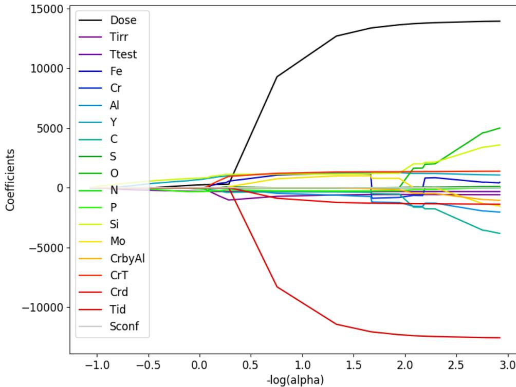
**Figure 5. Coefficients fitting path of the lasso-LARS algorithm applied to FeCrAl alloy data for yield stress. Large positive coefficients indicate an embrittling effect, while large negative coefficients indicate a softening or toughening effect.**
