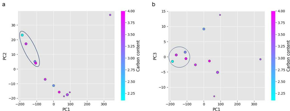
**Figure 11. Results of principal component analysis on grey cast iron images converted to n-point statistic representations. Circled points correspond to images of unetched samples.**
