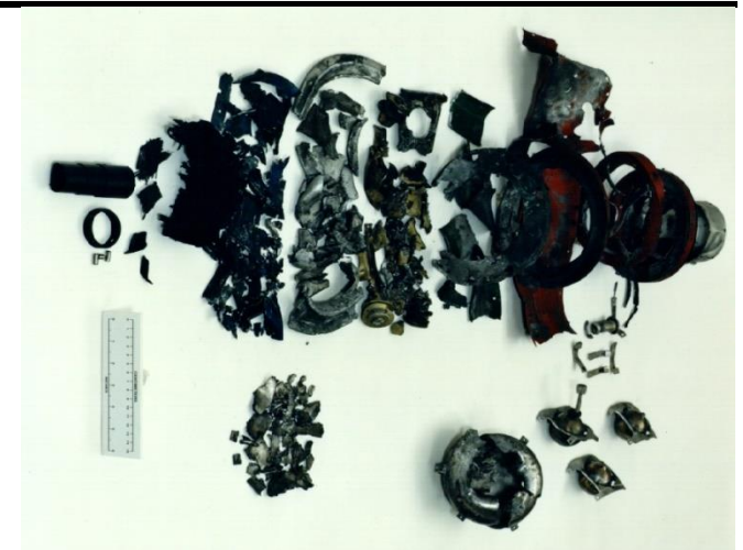
Typical debris from a satellite breakup (DoD SOCIT Tests, 1993).
