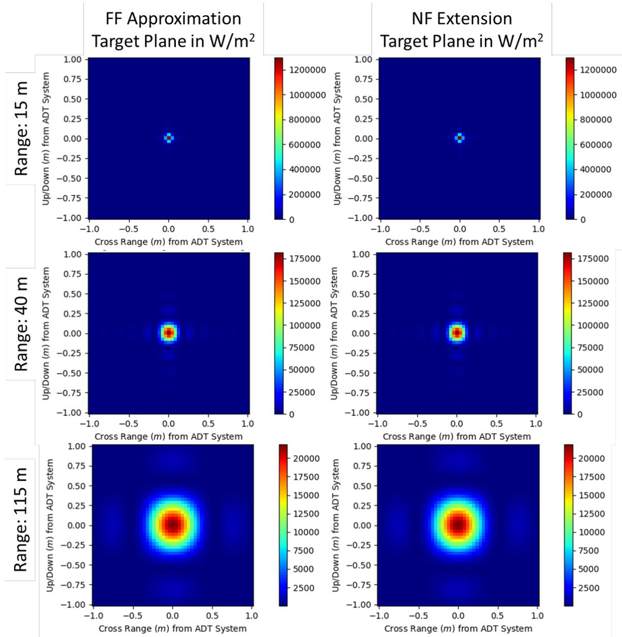
**Figure 4: Comparison of the incident beam profiles in the target plane as estimated by our FF (left column) and NF (right column) models at 15 m, 40 m, and 115 m down-range of a variable-focus system.**
