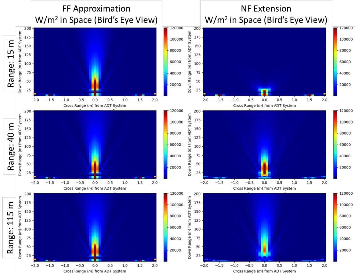
**Figure 6: Comparison of the incident beam profiles in the down-range, cross-range plane (“bird’s eye” view) as estimated by our FF and NF models at 15 m, 40 m, and 115 m down-range of a variable-focus system.**
