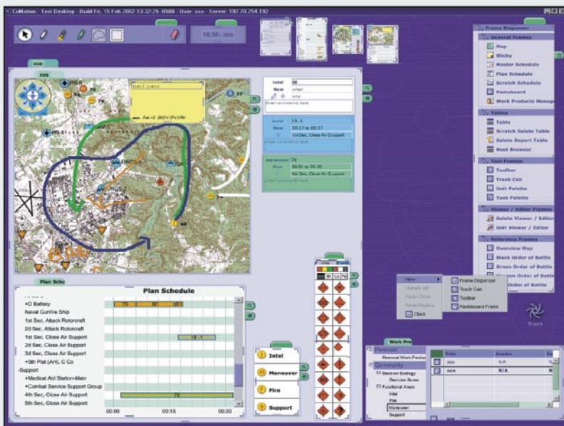
Figure 1. Typical CPOF Commander's Screen includes annotated map with Task Ink and Task Icons, Task Boxes, Planning Schedules, Tools, and Palettes.
